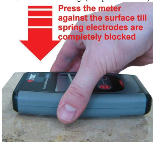
It is recommended to repeat the measurement in a few points situated next to each other as humidity has a tendency of uneven distribution. If the measurements vary, only the highest outcomes should be used.
