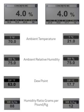
To change temperature between °C and °F and the Humidity Ratio between g/kg and grains/lb, press the button to go the Main Menu; scroll down and select 'TEMPERATURE SCALE' with the button, scroll and select with the button; and press the button to return to the main screen.
